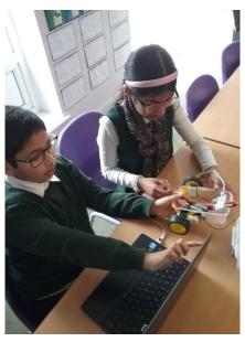
This week in D&T, Year 5 have connected two geared motors to their crumble controller. They then created programs to make a simple buggy move. To do this, the children had to make the code, run the code, disconnect the USB lead from crumble, put the buggy on the floor and turn the battery pack on.
